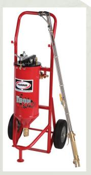
Iron Powder Dispenser (Ours also had 4, 100 lb O<sub>2</sub> tanks and 1, 50 lb tank of acetylene attached)
